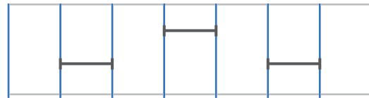
Two horizontal braces every two bays
