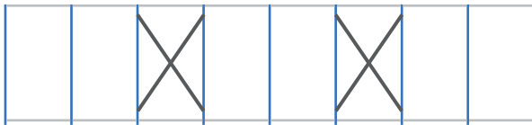
One cross brace every four bays
